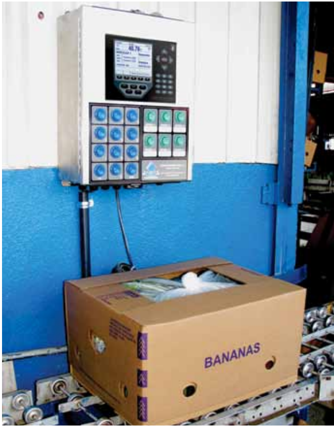
Rep. Roma's BANACHECK checkweigher uses oversized buttons for quickly switching from one grade of product to another.
