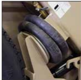
Transport Mode: When transporting, air bags are inflated and load cells put in transport mode, locking the system in place to prevent damage to the load cells.
