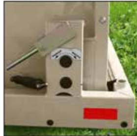
Transport Mode: When transporting, air bags are inflated and load cells put in transport mode, locking the system in place to prevent damage to the load cells.
