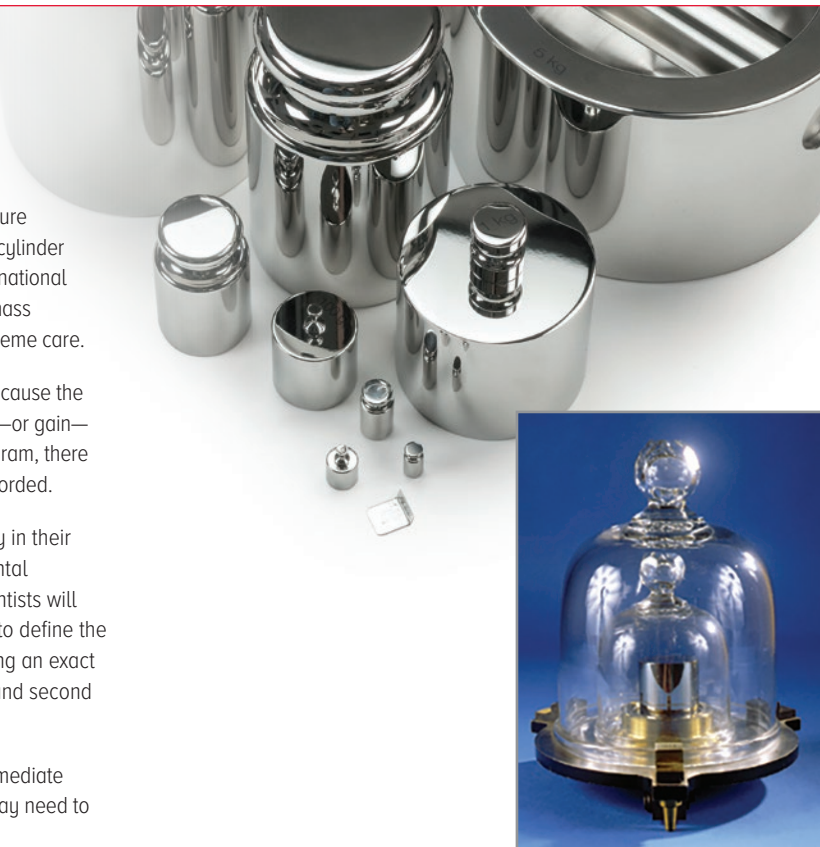
Up until the SI redefinition in 2019, the National Institute of Standards and Technology (NIST) housed and maintained America’s official mass standards. Pictured above, the K20 kilogram mass standard served as the primary prototype national standard.
