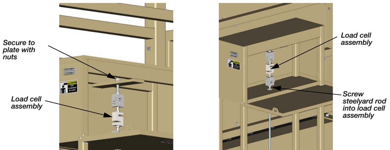
Figure 2-7. Load Cell Assembly
