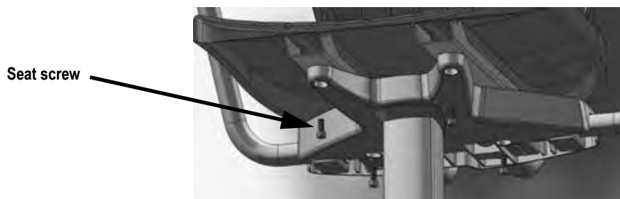
Figure 2-13. Secure Seat to the Scale Using Screws
