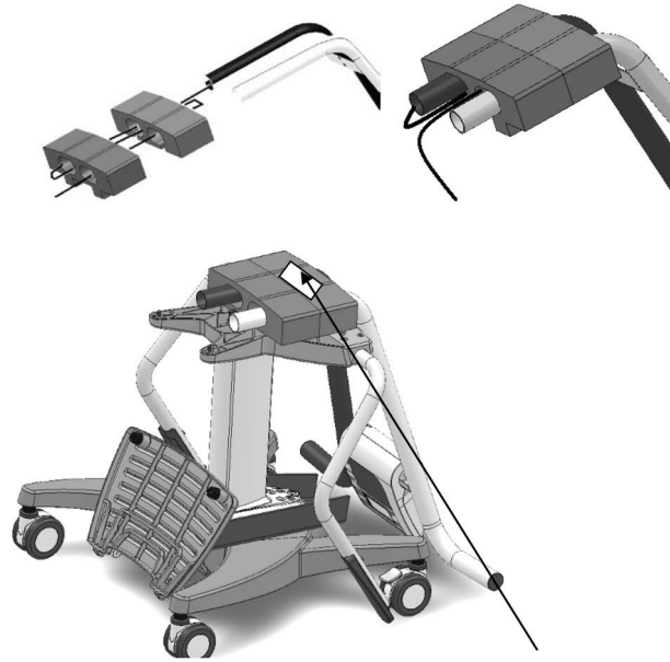
Figure 2-7. Remove Styrofoam Packing Pieces From Main Handle
