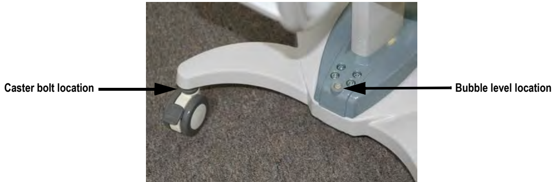
Figure 2-14. Bubble Indicates That The Scale is Level
