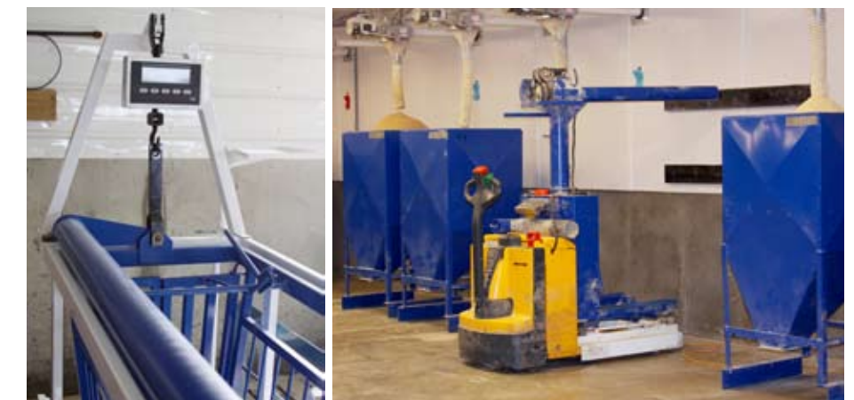
Mosdal teams the Rice Lake 390-DC to their custom equipment. The stainless steel enclosure can be washed down and the big display can be seen in dusty barns.
