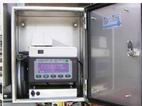
Rice Lake implemented custom software in the 520 indicator to compensate weight according to level.
