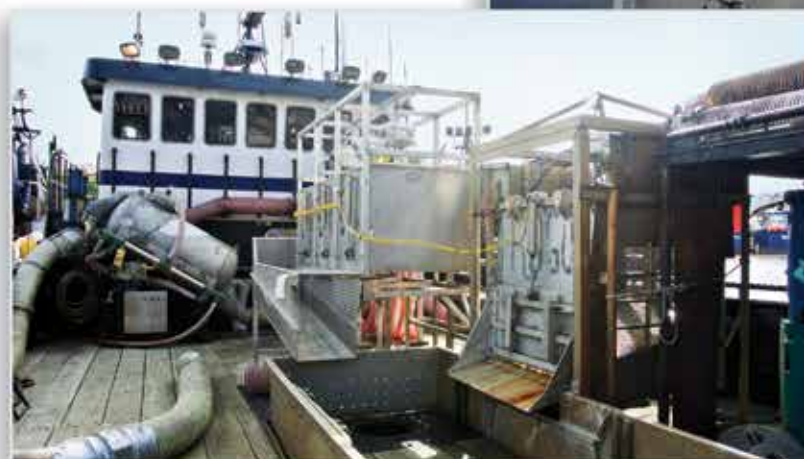
The Rogue is equipped with Port-A-Weighs and a vacuum suction system to transport the fish. Port-A-Weighs ensure an accurate weight despite the turbulent ocean waters.
