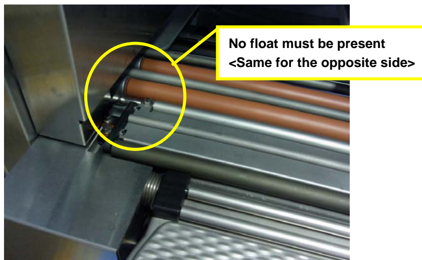
Picture 1: Heater guard
