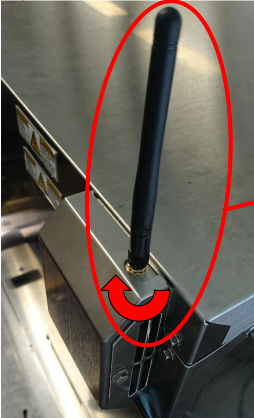
Step 12. Mount the Wi-PORT antenna.
