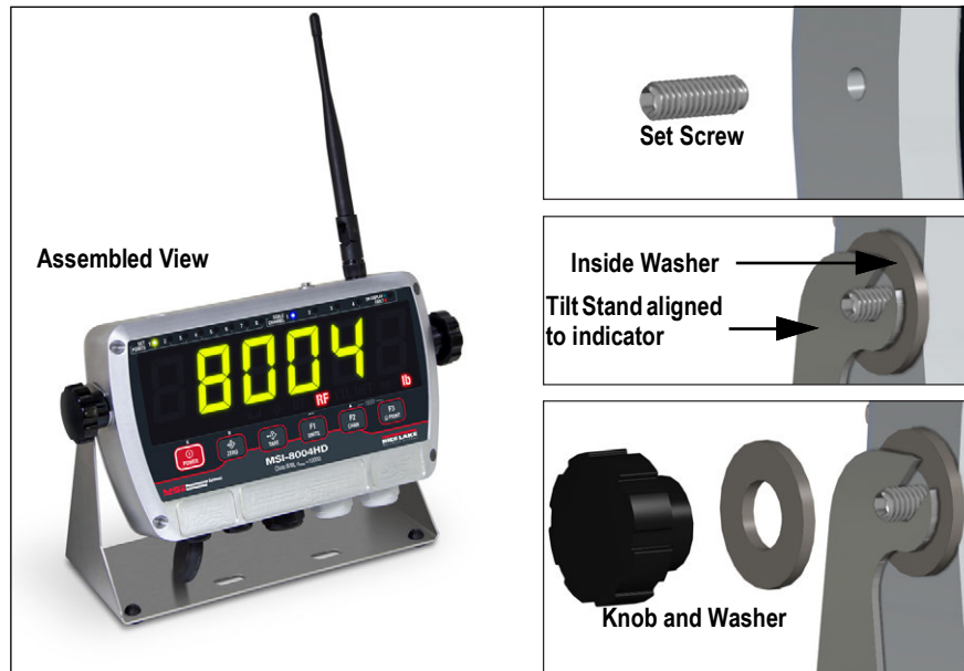
Figure 2-12. Install Tilt Stand
