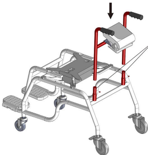
Figure 2-5. Insert Handle Assembly to Chair Frame
