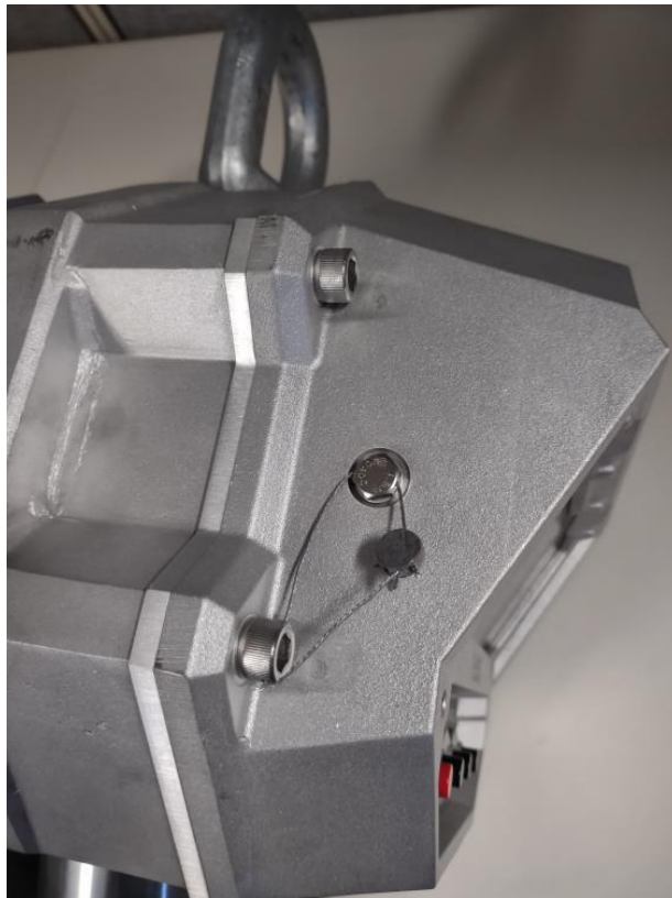
Typical Sealing / Scellage typique
