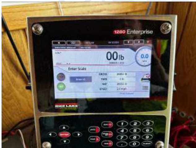
Indicator with WIM Application Operator's Screen
