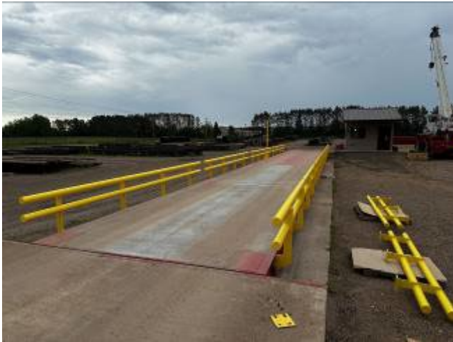
Weighing/Load Receiving Element showing Side Rails
