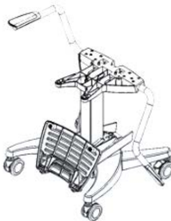
Figure 2-3. Rotate the Arm Rests
