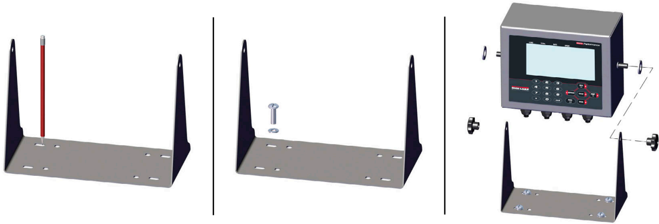
Figure 2-2. Mounting the 882D
