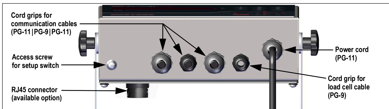
Figure 2-5. Recommended Cord Grip Assignments
