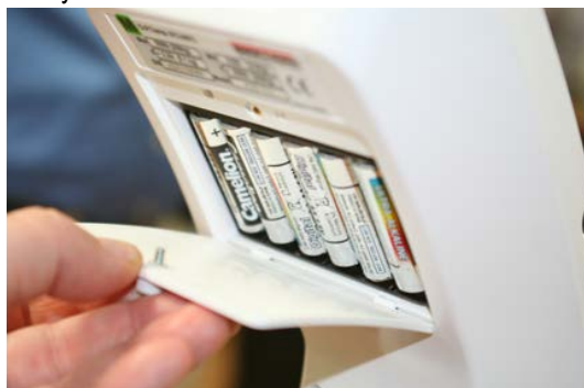
Figure 2-4. Batteries in Battery Chamber
