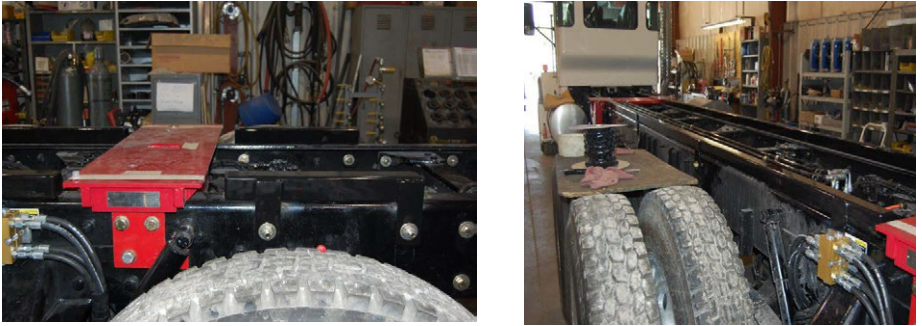
Figure 2-7. Simple Closed Square Tubing Support
