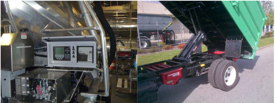
Kiosk at Rear of Tip Tank
