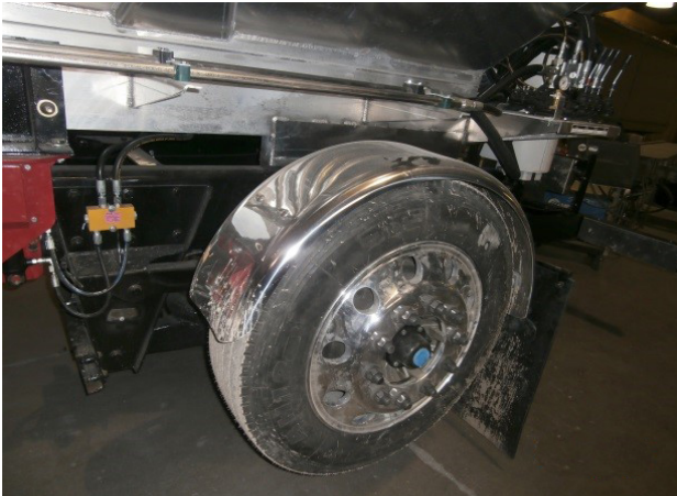
Figure 2-6. Support Spacer on an Aluminum Body
