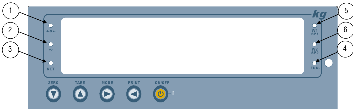
Figure 6.4 – Keys and indicators of the DGT60 front panel
