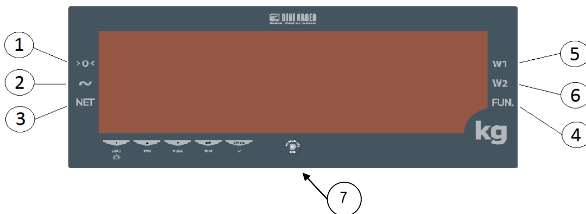
Figure 6.5 – Keys and indicators of the DGT100 front panel
