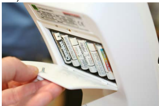
Figure 2-7. Batteries in Battery Chamber
