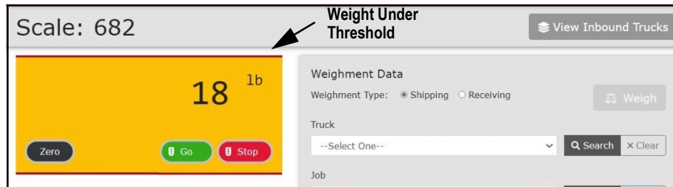
Figure 9-5. Weight Under Threshold
