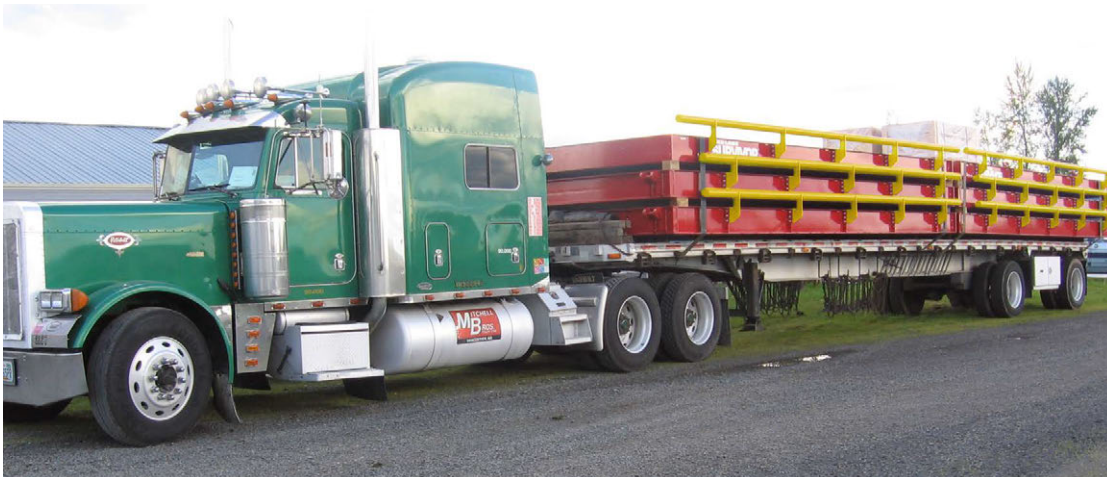
Figure 3-2. Weigh Modules Ready for Removal and Installation
