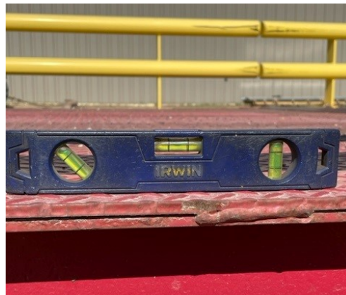
Figure 3-8. Check Weighbridge for Level
