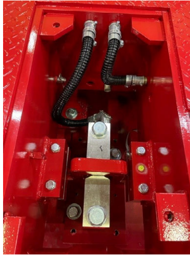
Figure 4-5. Load cell Access
