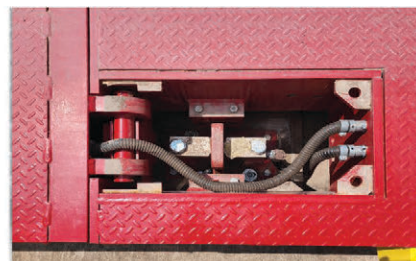
Figure 5-5. Conduit Connection Between Deck Modules
