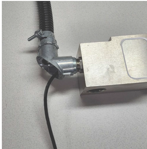
Figure 4-3. Installing 90° Fitting to Load Cell
