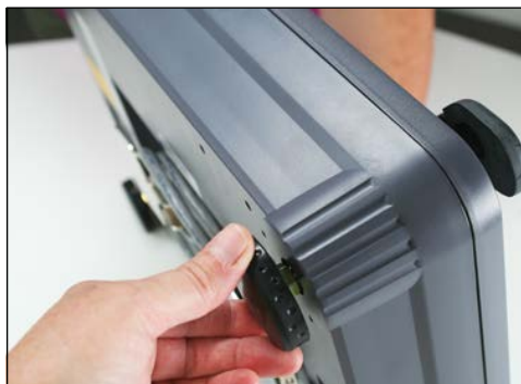
Figure 2-4. Adjust the Scale Base Feet
