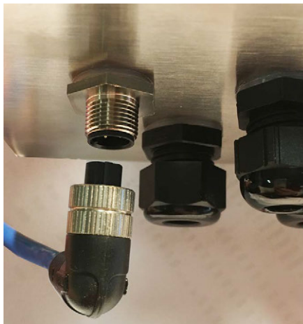
Figure 3. Cable Connection to the 882IS
