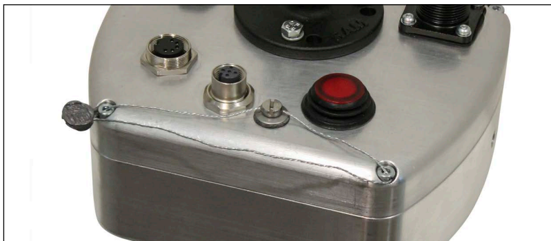
Figure 2-12. Sealing the Enclosure – No Access
