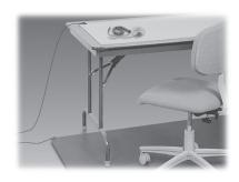
An absolute must for every workbench, this kit includes a 3-layer  $2 \times 4$  ft table mat,  $4 \times 6$  ft floor mat, ground cord and adjustable wrist strap. Designed specifically for energized circuit work, the static control table and floor mat provide superior protection against ESD.
