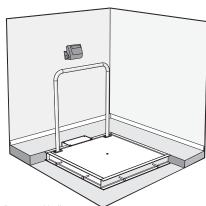
Wall mounted indicator, cable enclosed in customer supplied conduit.
