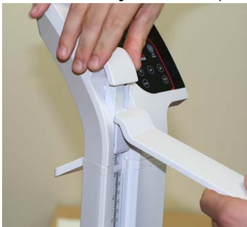
Figure 2-7. Height Rod Assembly
