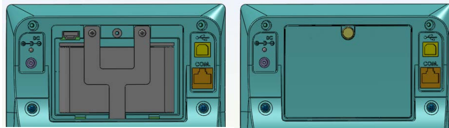
Figure 3-3. Rechargeable Battery Without Cover (left) and With Cover (right)
