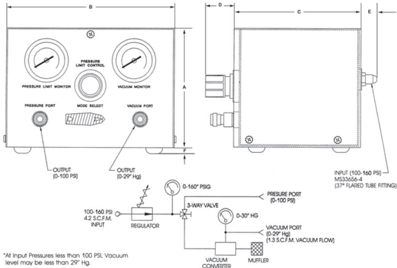
\*At Input Pressures less than 100 PSI, Vacuum level may be less than 29" Hg.
