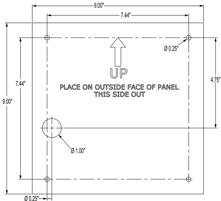
Figure 2-16. Panel Mount with Keypad Dimensions
