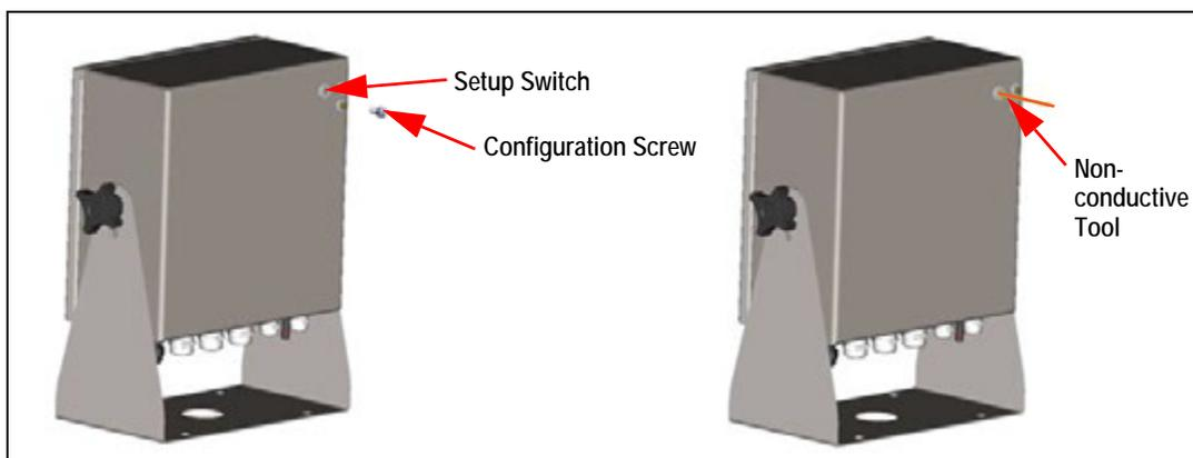
Figure 3-1. Setup Switch Location (Universal Enclosure)
