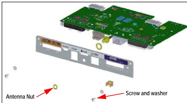
Figure 2-34. CPU Board and Face Plate
