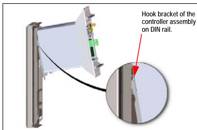
Figure 2-21. Hook Bracket on DIN Rail
