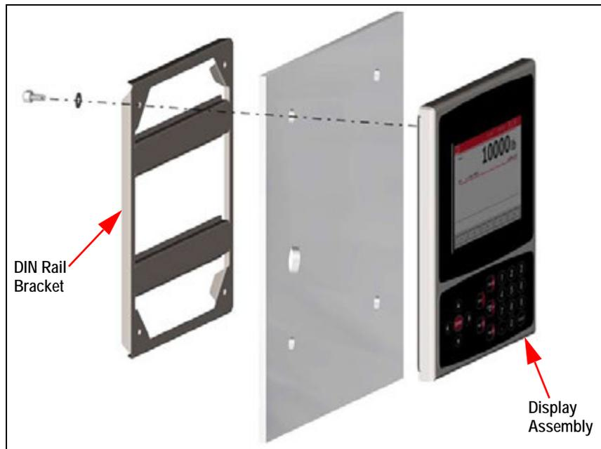
Figure 2-19. Panel Enclosure Mounting
