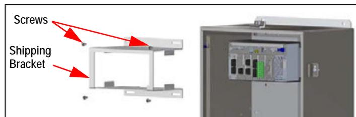
Figure 2-9. Remove Shipping Bracket
