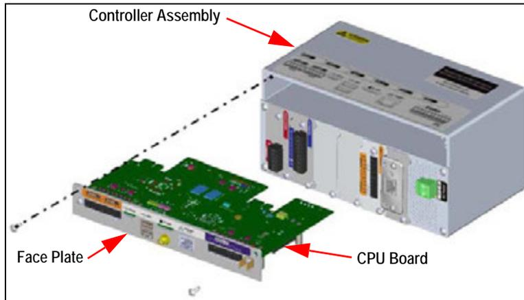
Figure 2-33. Remove CPU Board
