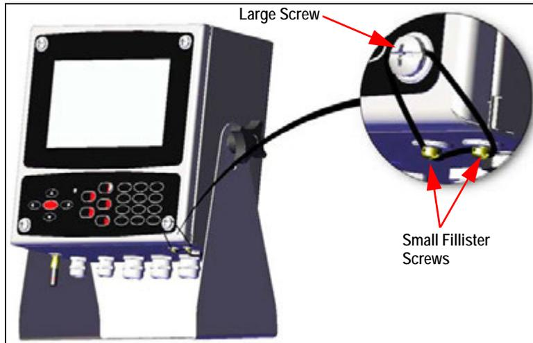
Figure 2-7. Seal the Front Door (Universal Mount)
