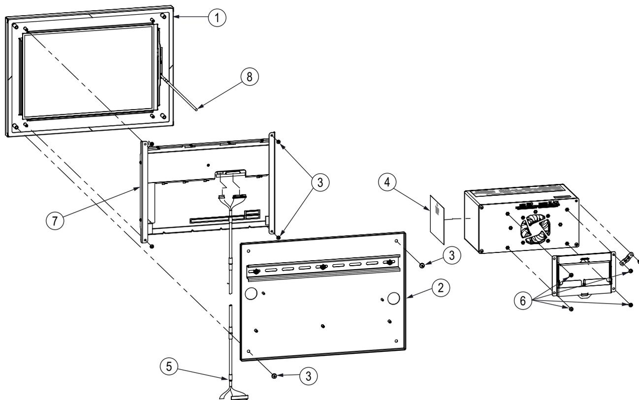
Figure 2-43. Panel Mount Touch Screen – 12" Repair Parts
