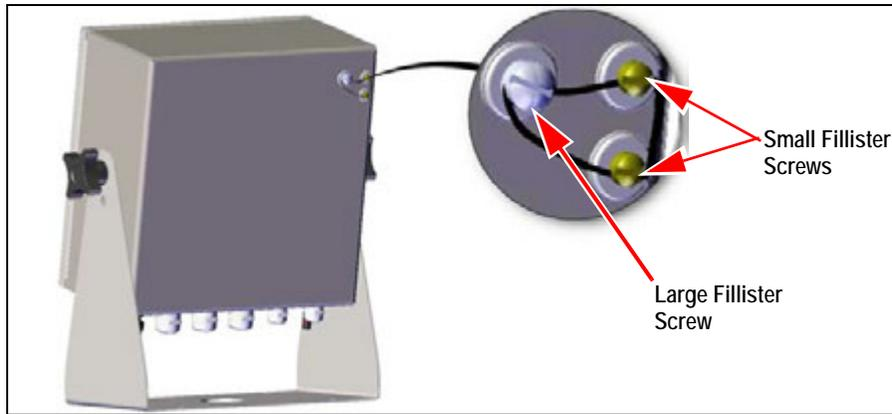
Figure 2-6. Seal the Setup Switch (Universal Mount)
