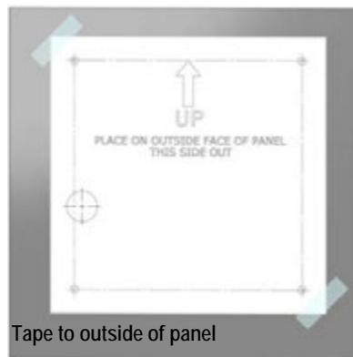
Figure 2-15. Mark and Drill Holes for Panel
