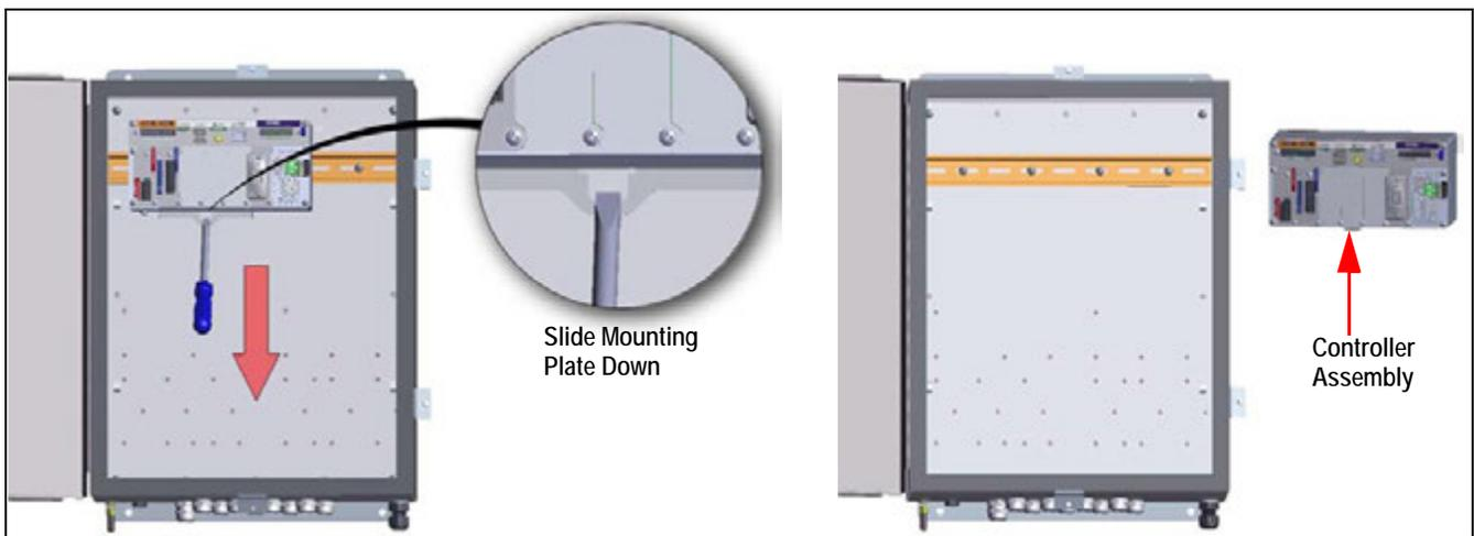
Figure 2-11. Remove Controller Assembly - Wall Mount
