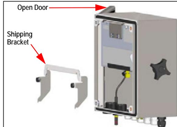
Figure 2-2. Remove Shipping Bracket
