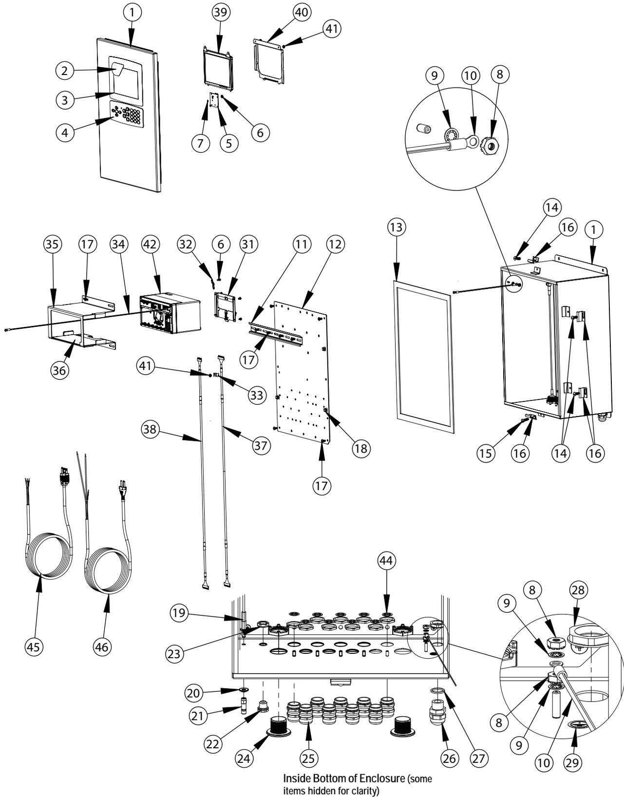
Figure 2-41. Wall Mount Repair Parts
