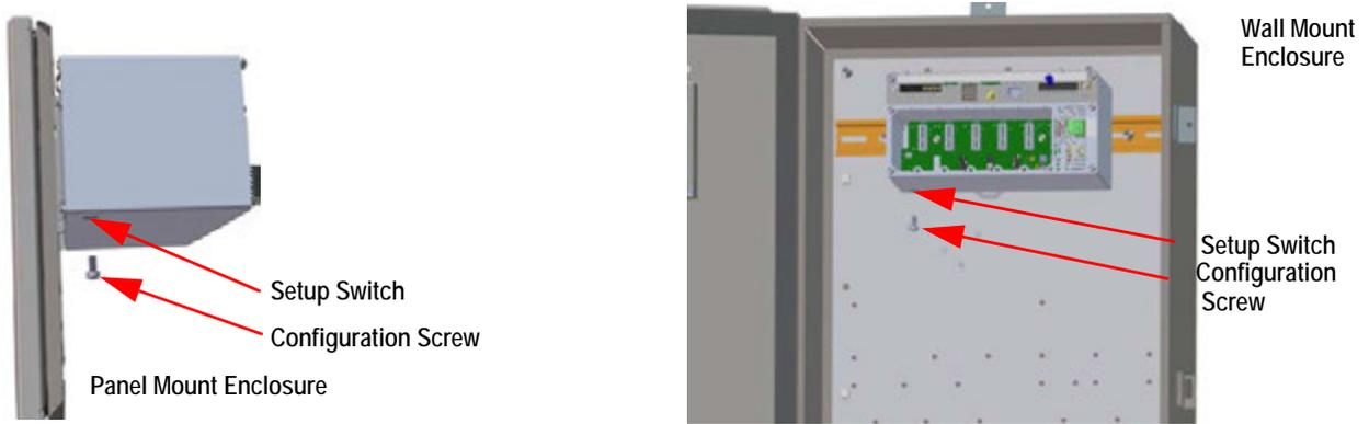
Figure 3-2. Setup Switch Locations (Panel/Wall Mount Enclosures)
