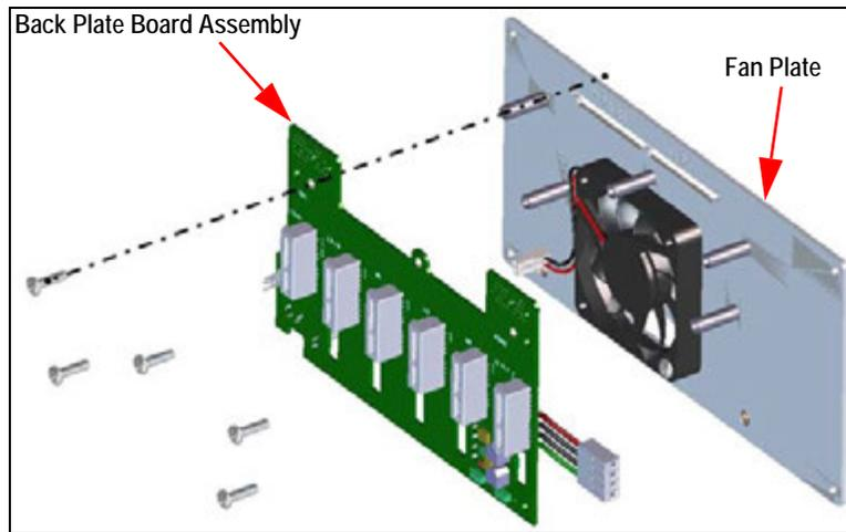
Figure 2-36. Remove Back Plate Board Assembly
