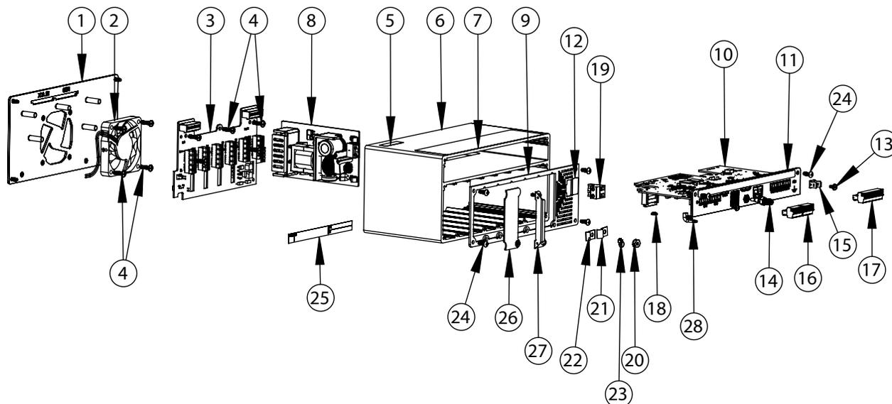
Figure 2-38. Controller Assembly Repair Parts
