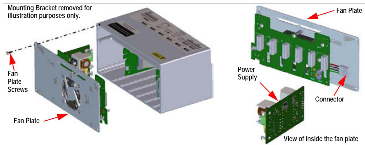
Figure 2-35. Remove Power Supply
