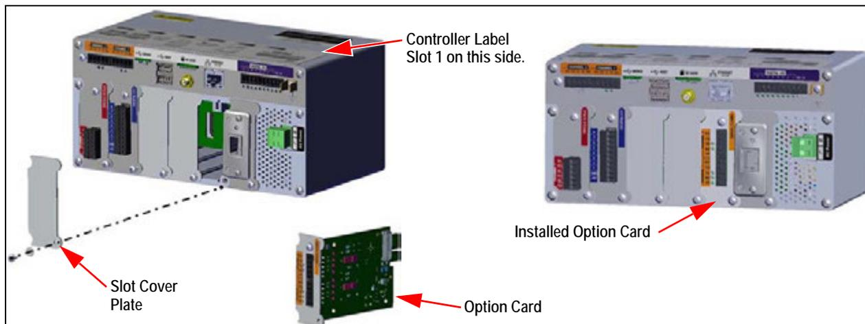
Figure 2-25. Option Card Installation
