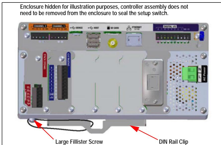
Figure 2-12. Seal the Setup Switch
