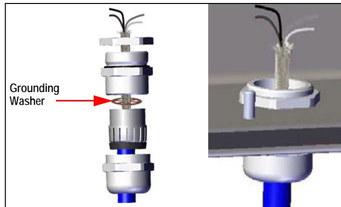
Figure 2-27. Universal and Wall Enclosure Grounding
