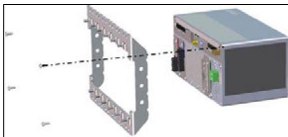
Figure 2-20. Grounding Bus Bar Installation
