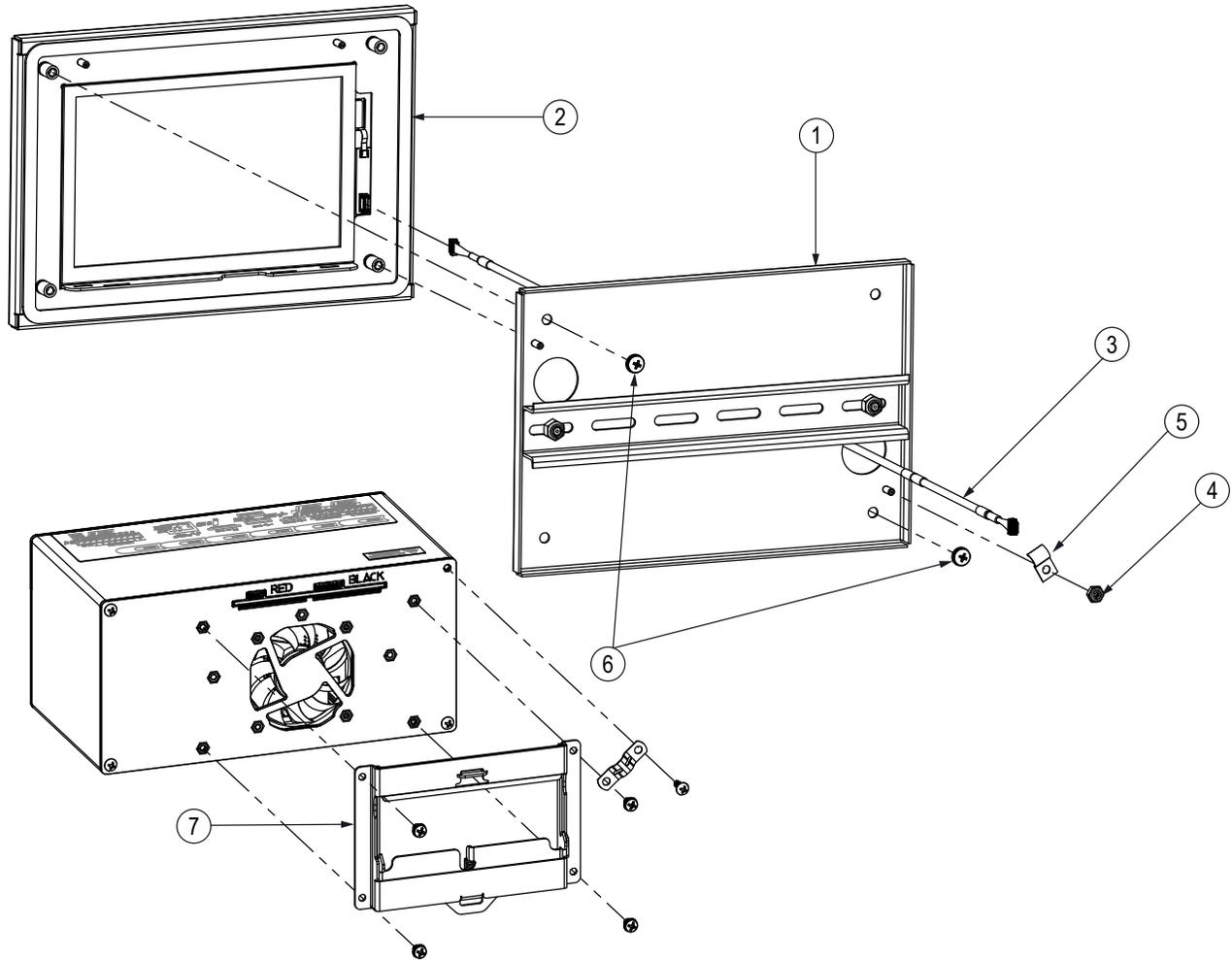
Figure 2-42. Panel Mount Touch Screen – 7" Repair Parts
