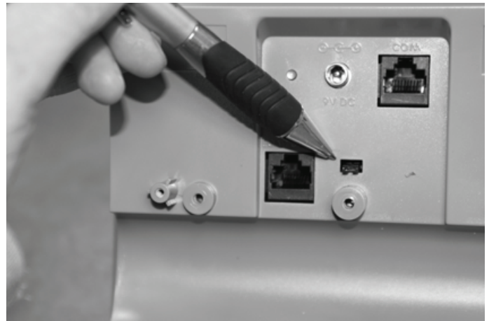
Remove jumper to gain access to configuration and calibration modes
