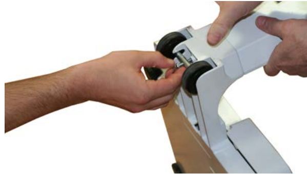
Figure 2-3. Attach Wheel Assembly
