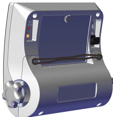
Figure 6-2. Wire Sealing Location
