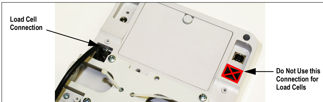
Figure 2-4. Load Cell Connection Point
