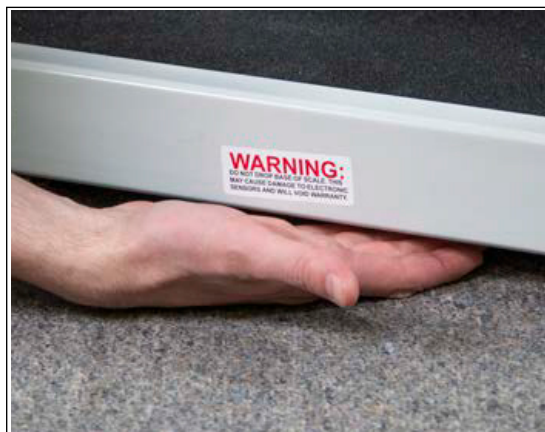
Figure 2-5. Scale Base Clearance
