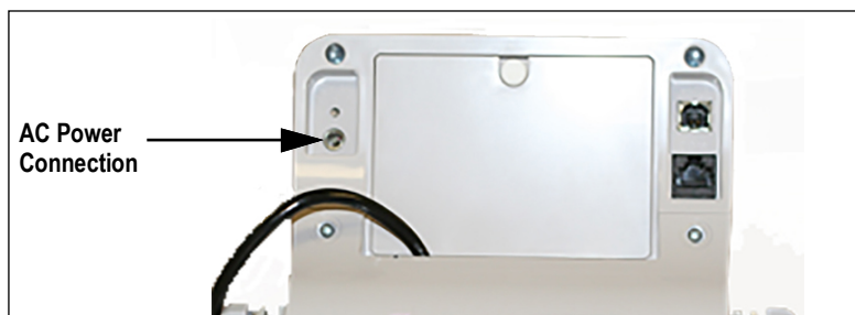
Figure 2-11. Power Connection Site
