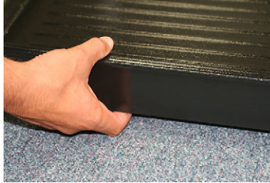
Figure 2-2. Clearance Between Scale Base and Floor
