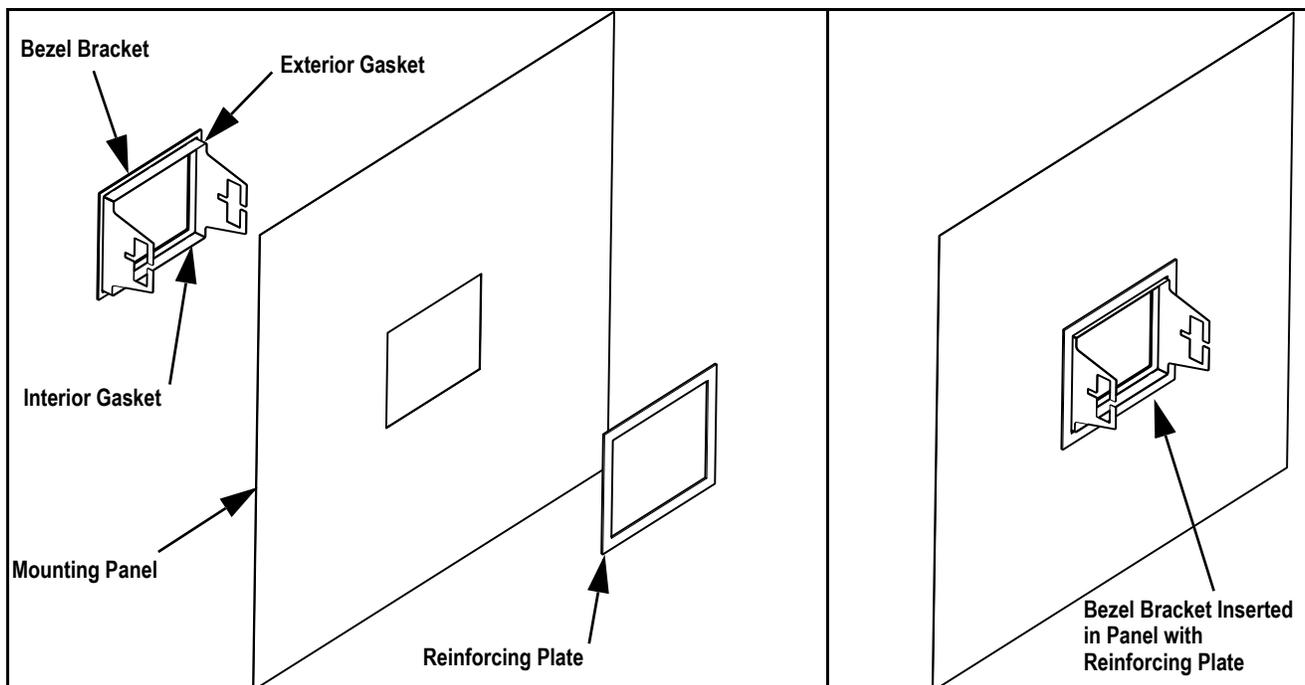
Figure 3. Insert Bezel Bracket
