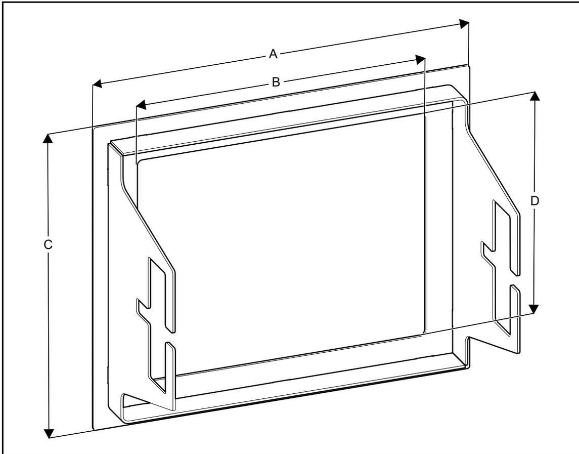
Figure 6. Bezel Bracket Dimension Diagram
