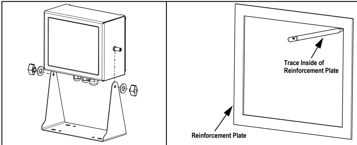
Figure 2. Remove Tilt Stand and Trace Cutout Lines
