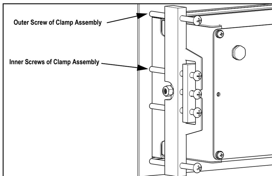
Figure 5. Tighten Clamp Assembly
