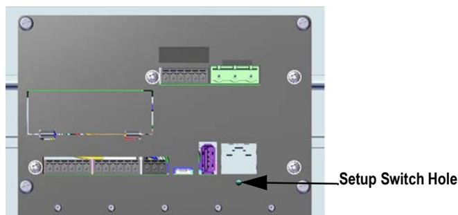
Figure 3. Setup and Configuration Switch Hole
