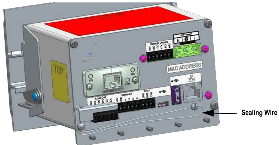
Figure 2-29. Install Sealing Wire
