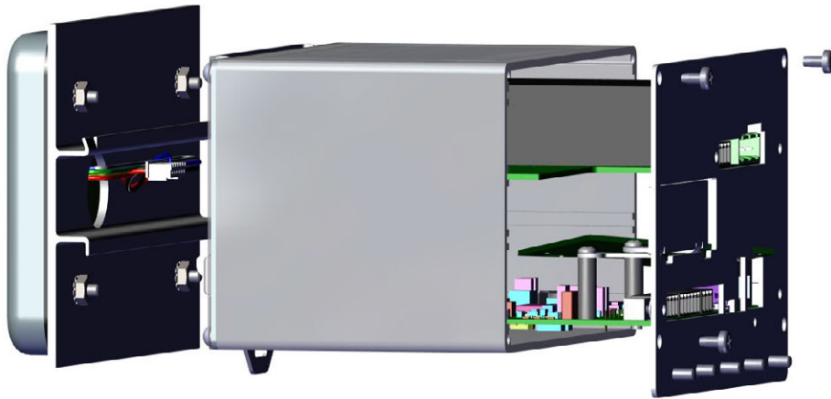
Figure 2-9. Remove Controller Assembly Backplate
