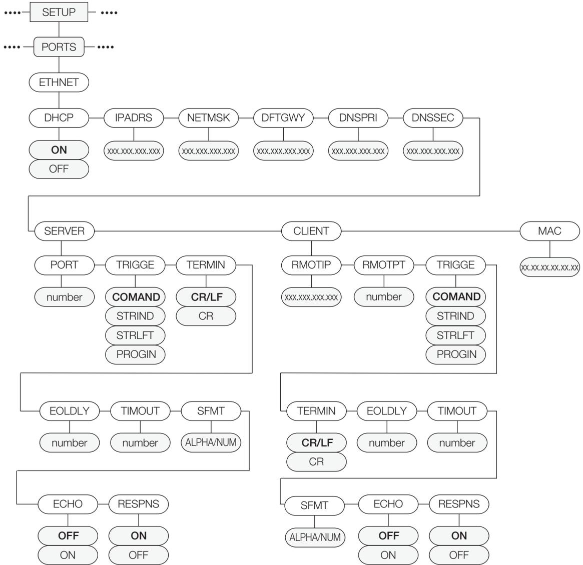
Figure 3-12. Ethernet Menu Structure
