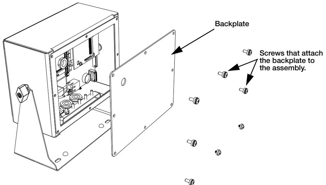
Figure 2-14. Remove Universal Mount Backplate
