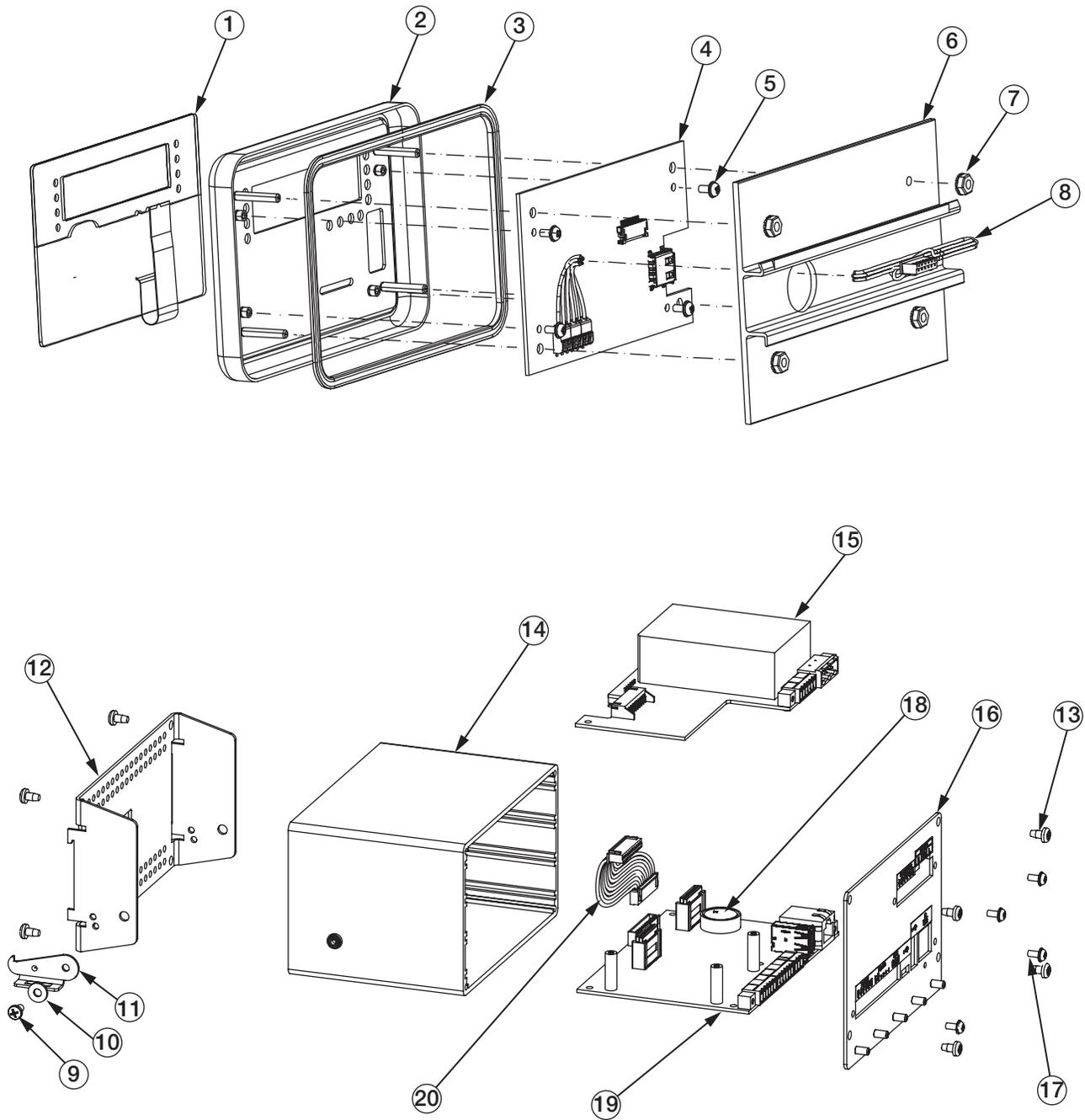
Figure 2-24. 880 Indicator Parts Illustration
