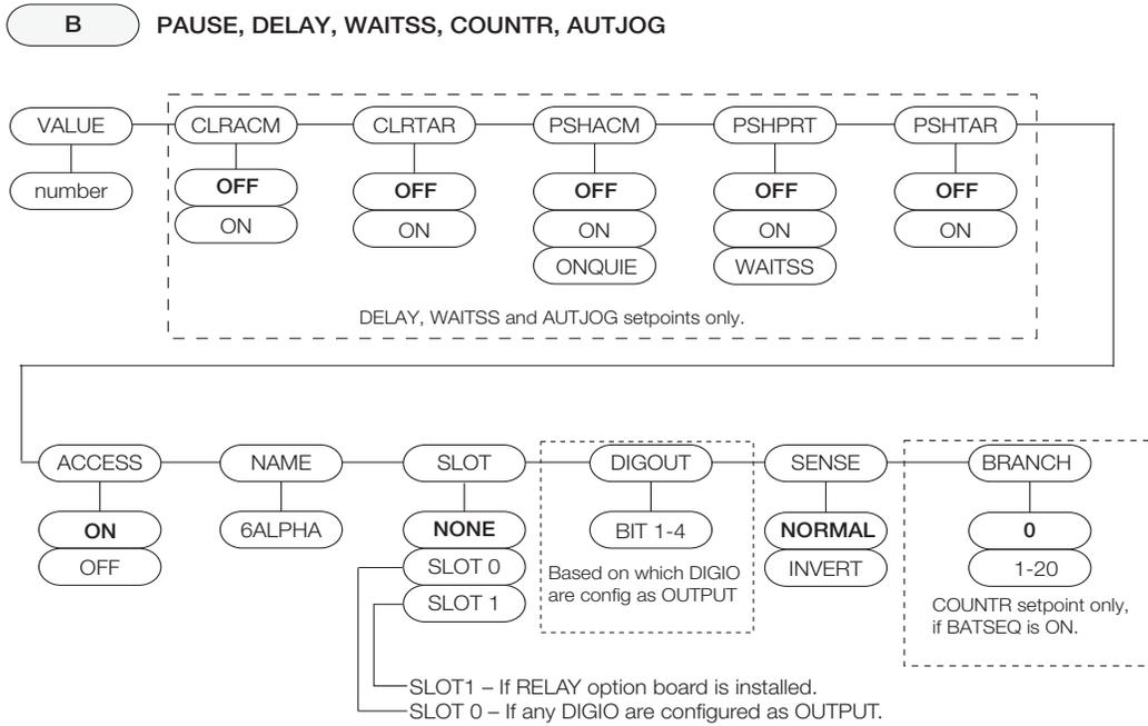
Figure 3-17. Setpoint Menu Structure – Layout B
