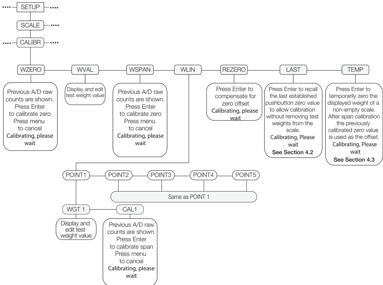
Figure 4-1. Calibration (CALIBR) Menu
