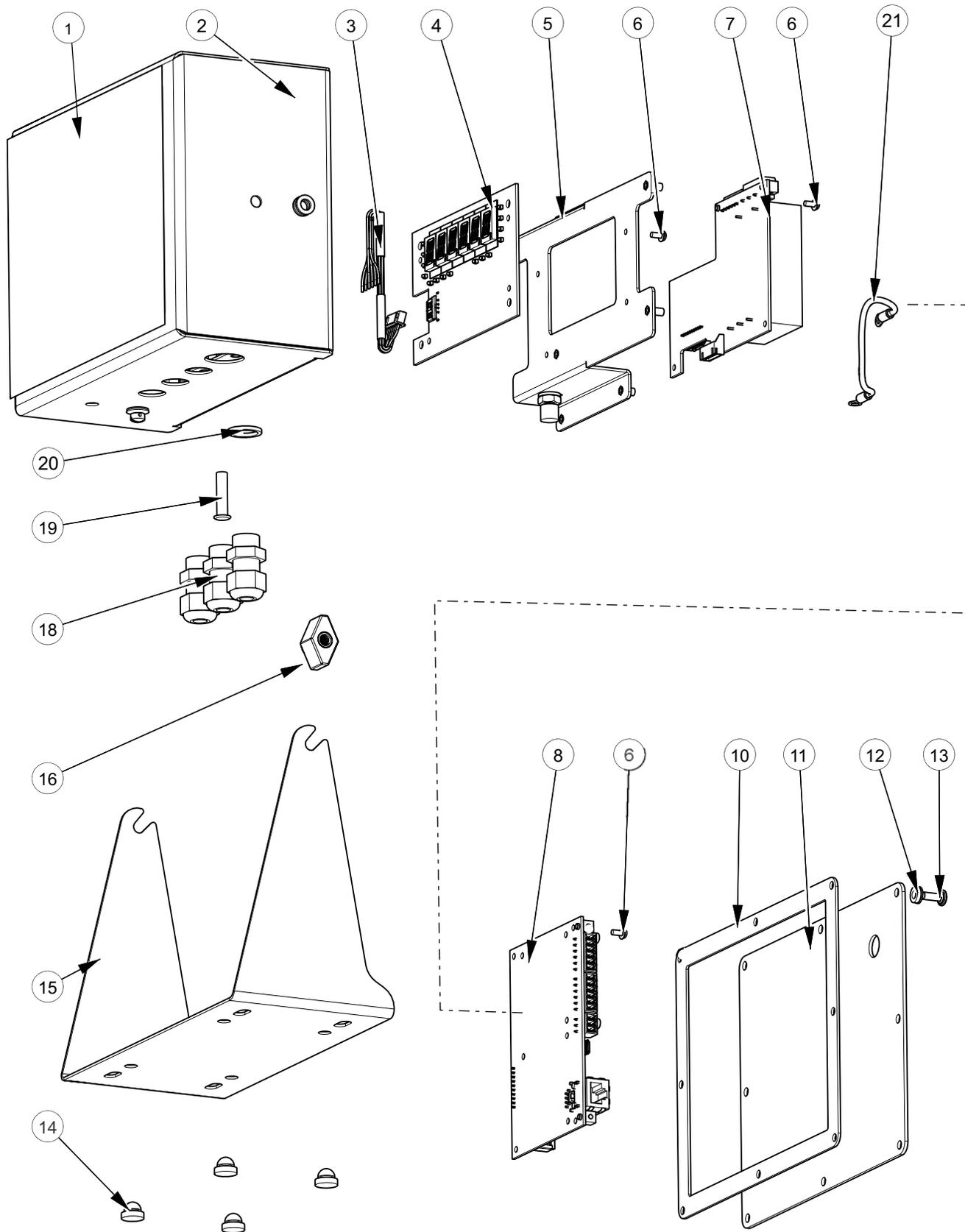
Figure 2-25. 880 Indicator Universal Mount Repair Parts Drawing
