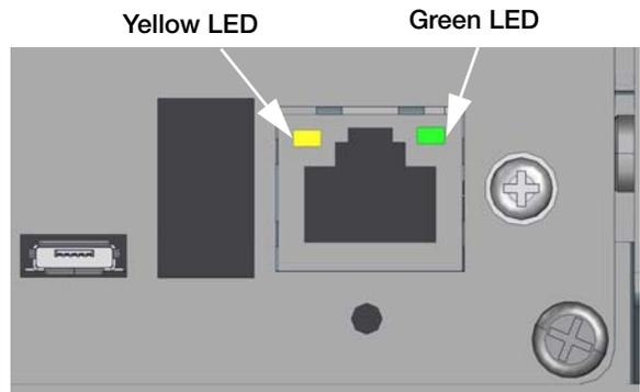
Figure 2-18. RJ45 Ethernet Jack – Panel Mount
