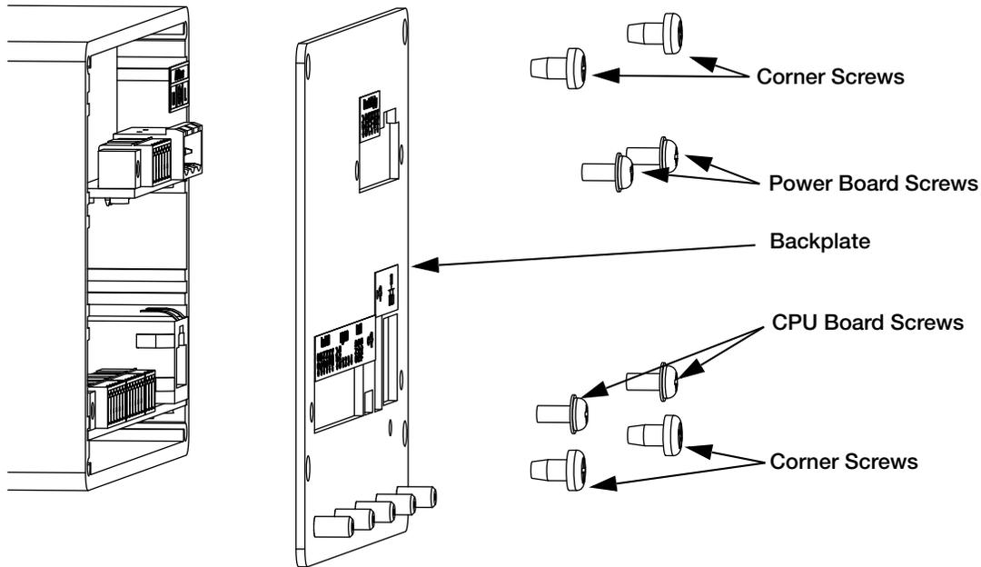
Figure 2-8. Remove Controller Assembly Backplate
