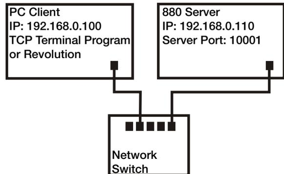
*Figure 9-2. Connection from PC to 880 Ethernet Through a Network Switch or Router*
