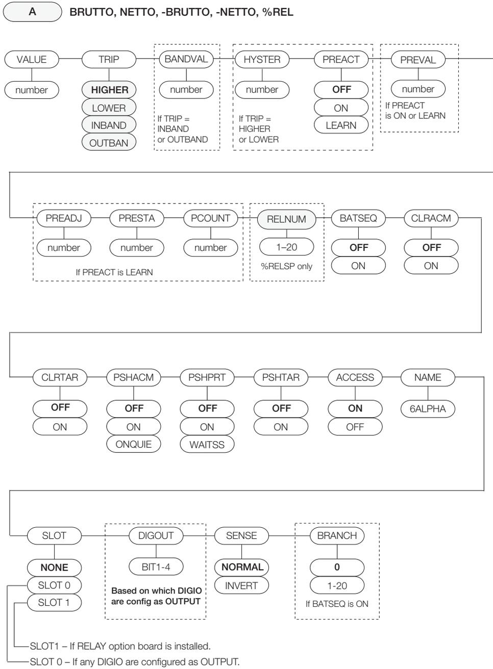
Figure 3-16. Setpoint Menu Structure – Layout A
