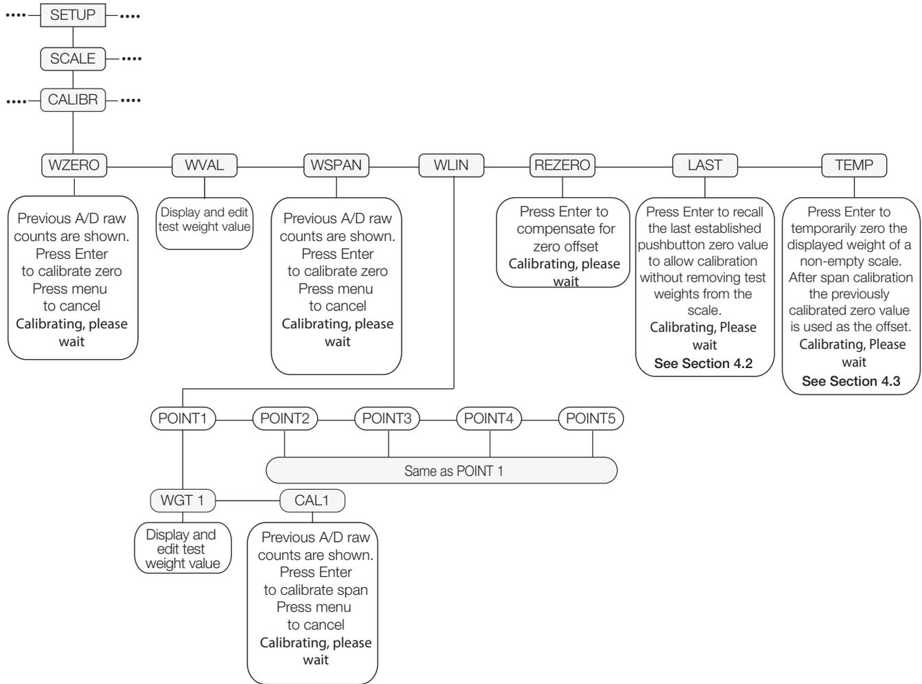
Figure 3-7. Calibration Menu Structure
