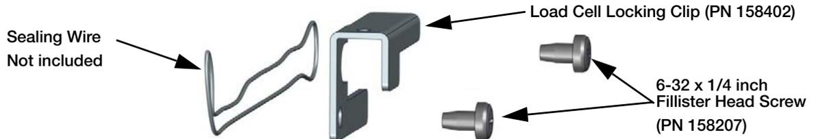
Figure 2-20. Sealing Components
