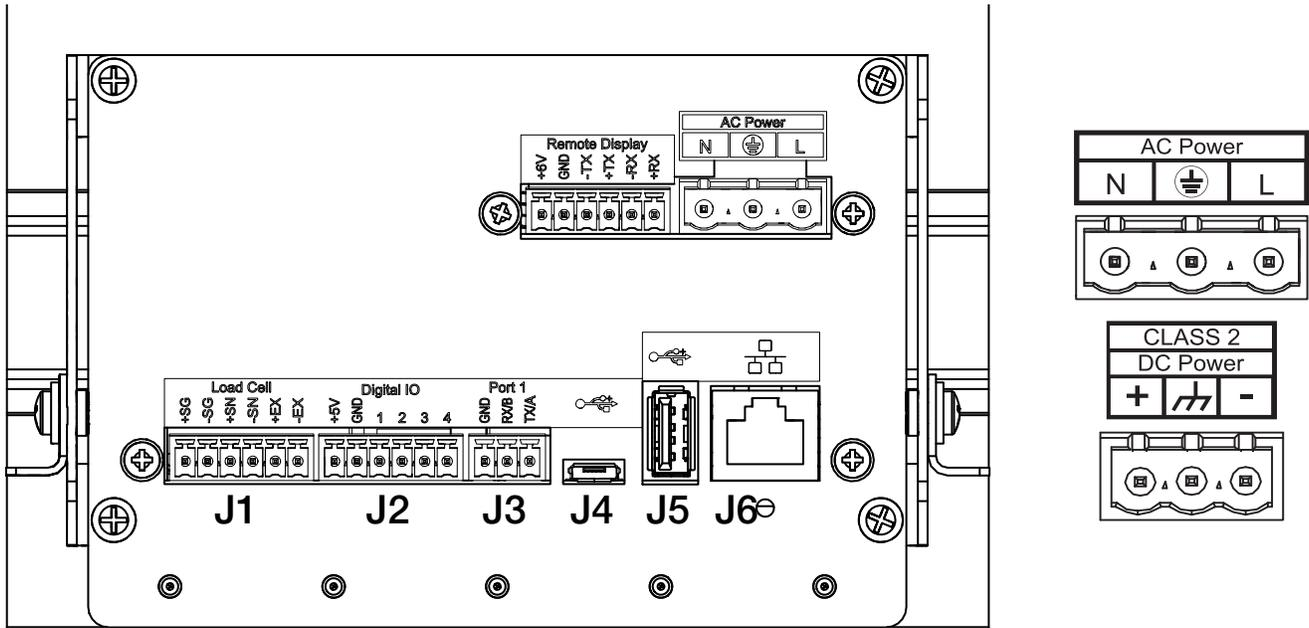
Figure 2-17. Power Connection Location
