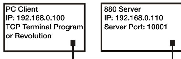
Figure 9-1. Direct Connection from PC to 880 Ethernet
