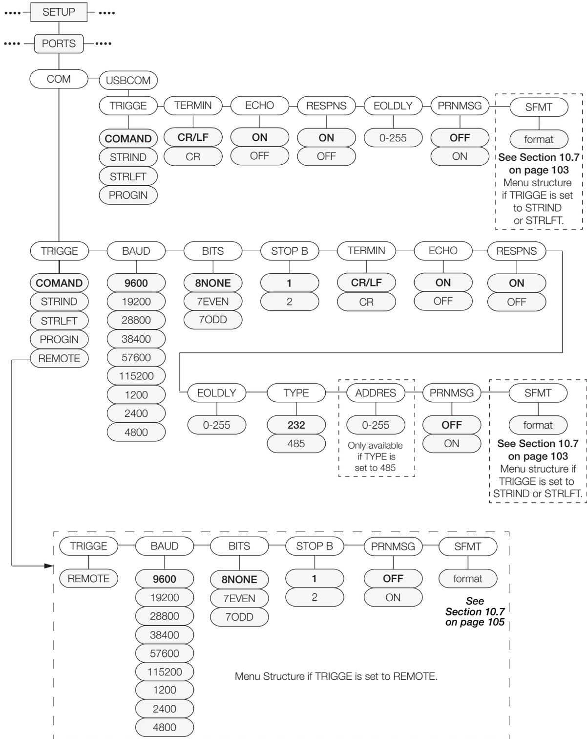
Figure 3-11. Com and USBCOM Menu Structure
