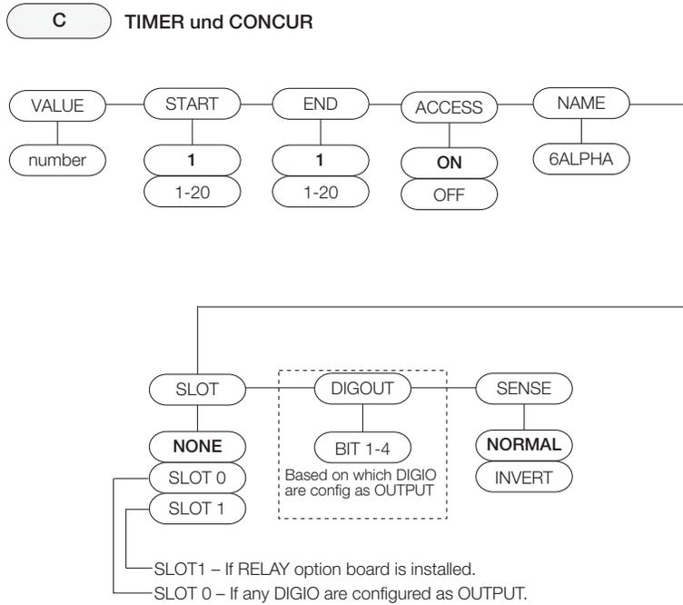
Figure 3-18. Setpoint Menu Structure – Layout C
