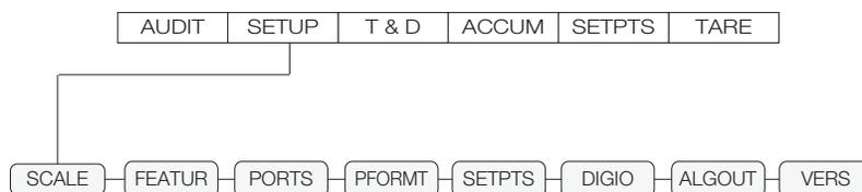
Figure 3-4. Setup Menu Structure
