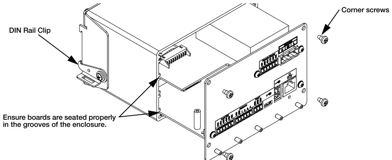
Figure 2-12. Boards Installed in Controller Assembly Enclosure
