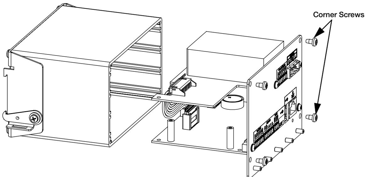
Figure 2-10. Remove Backplate With Boards
