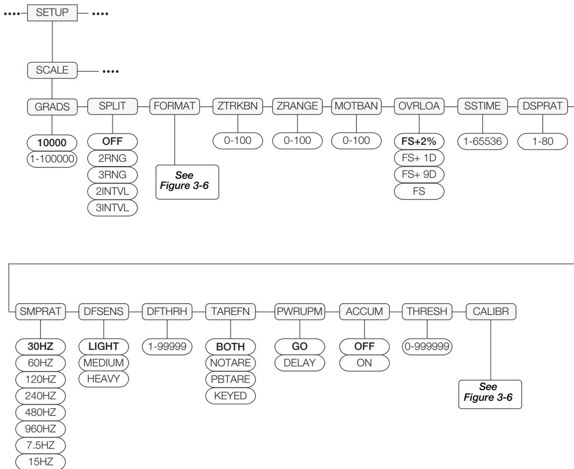
Figure 3-5. Scale Menu Structure
