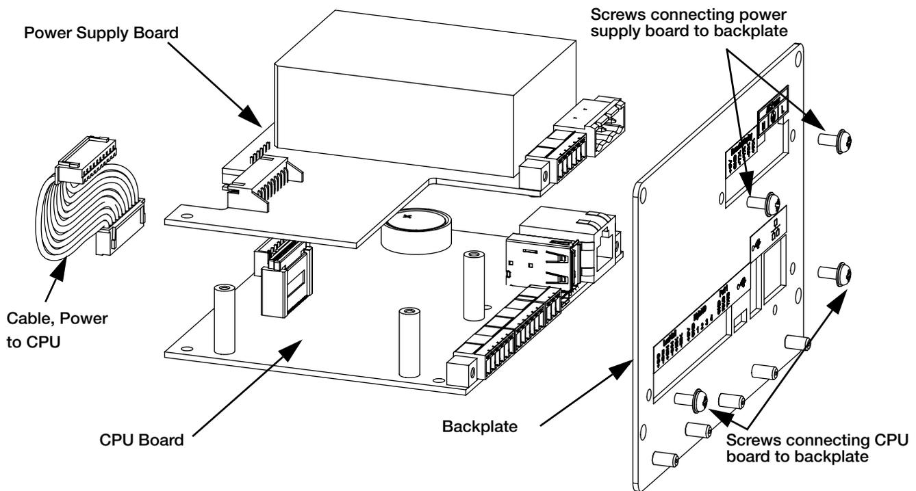
Figure 2-11. Boards Removed from Enclosure
