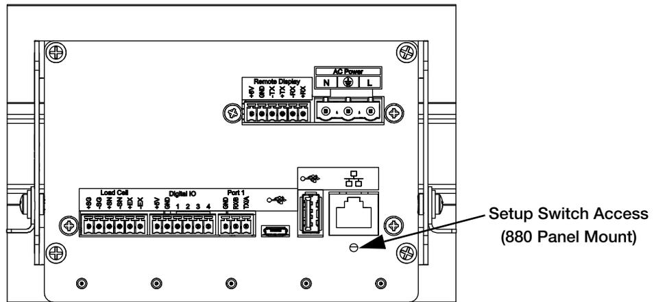
Figure 3-1. Back View – Setup Switch Access
