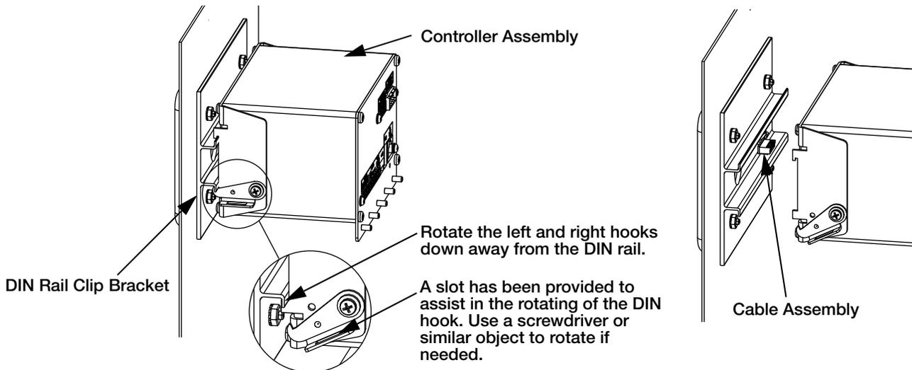
Figure 2-7. Remove Controller Assembly
