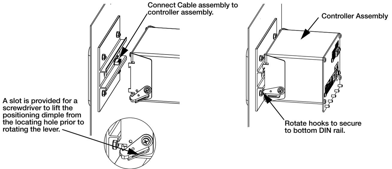
Figure 2-4. Install Controller Assembly
