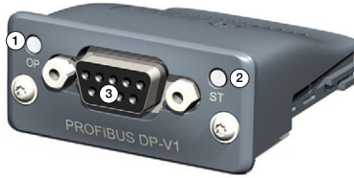
Figure 2-5. PROFIBUS DP Module
