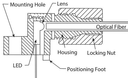
Figure 3. Fiber Optics Connector
