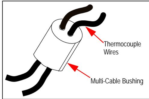
Figure 3. Multi-Cable Bushing
