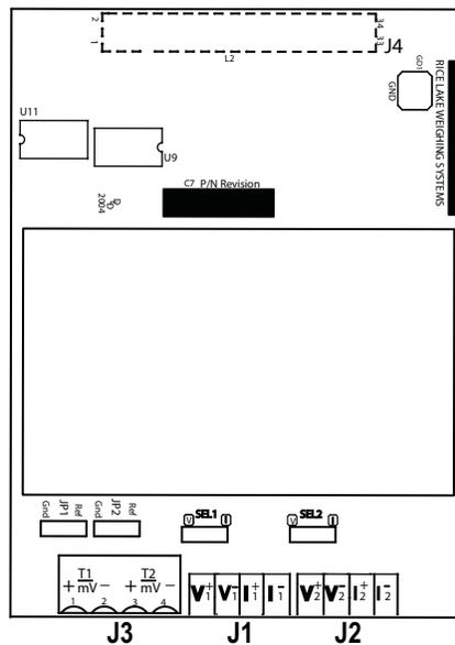
Figure 1. Dual Analog Input Card w/ Thermal Coupler
