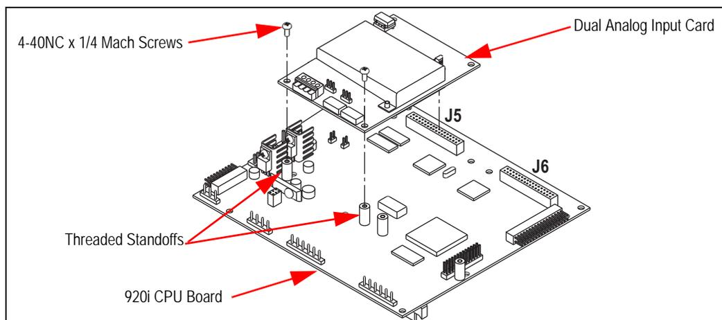
Figure 2. Dual Channel Analog Input Card with Thermocouple Input (PN 87697)
