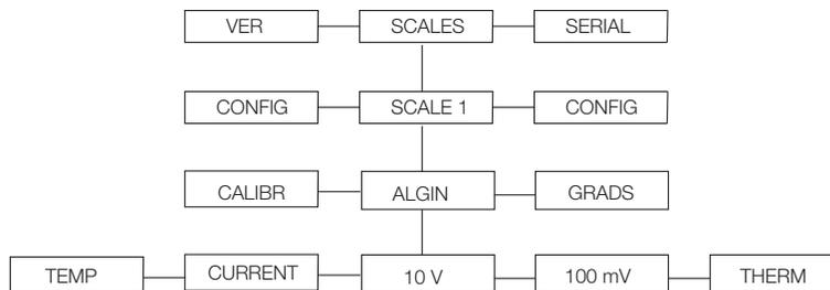
Figure 12. 0-10 V and 0-100 mV Analog Input Menus.
