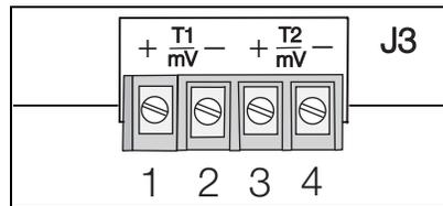
Figure 4. J3 – Thermocouple Wiring
