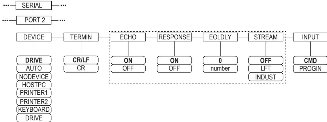
Figure 4-11. Port 2 (with USB Interface Option) Menu Layout
