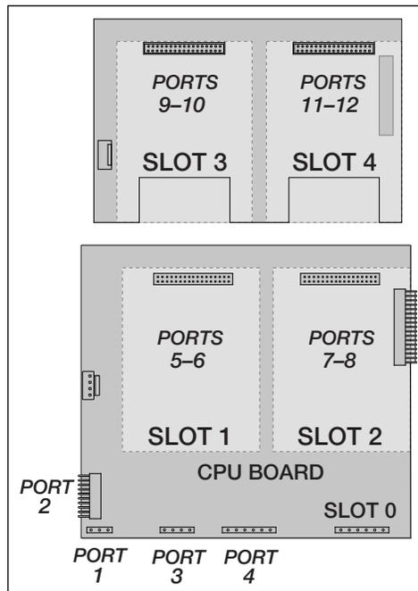
Figure 3-12. Serial Port Assignments, Two-Card Expansion Board
