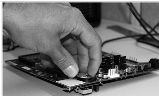
Figure 3-13. Battery Removal
