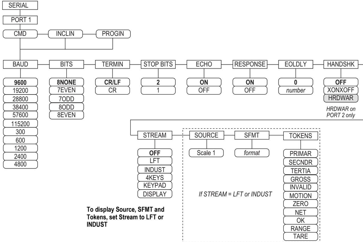
Figure 4-9. Serial Menu, Port 1 Menu Layout
