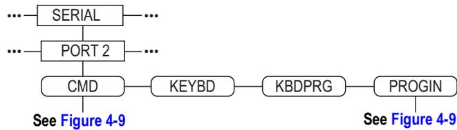
Figure 4-10. Port 2 (with Serial Interface Option) Menu Layout
