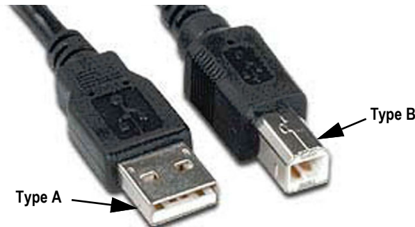
Figure 7-1. USB Connector Types
