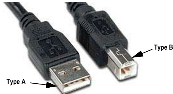
Figure 7-1. USB Connector Types
