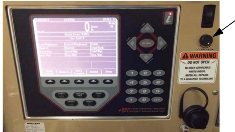
Figure 1. Contrast Control Potentiometer Installed
