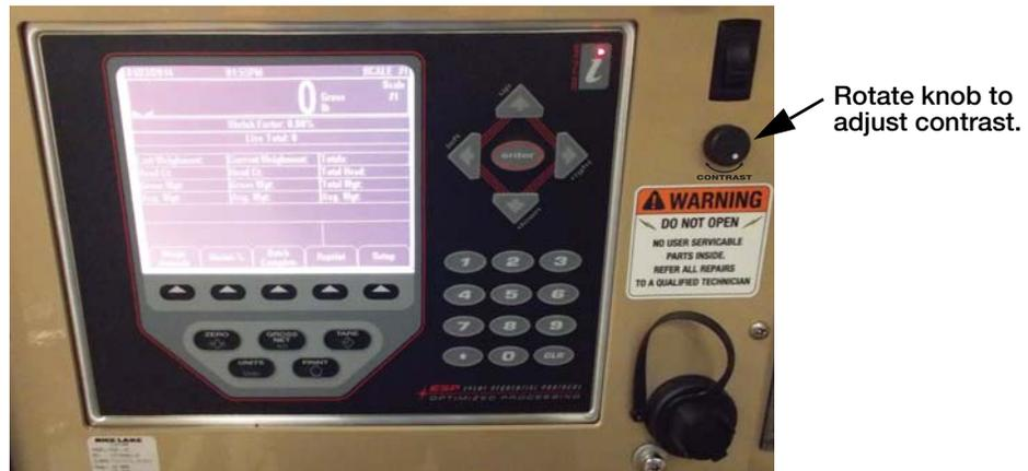
Figure 11. Contrast Control Potentiometer Installed
