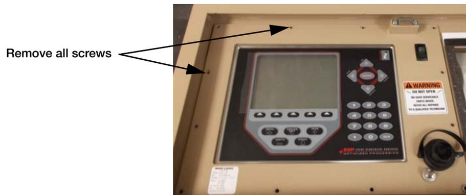
Figure 2. Remove Front Bezel
