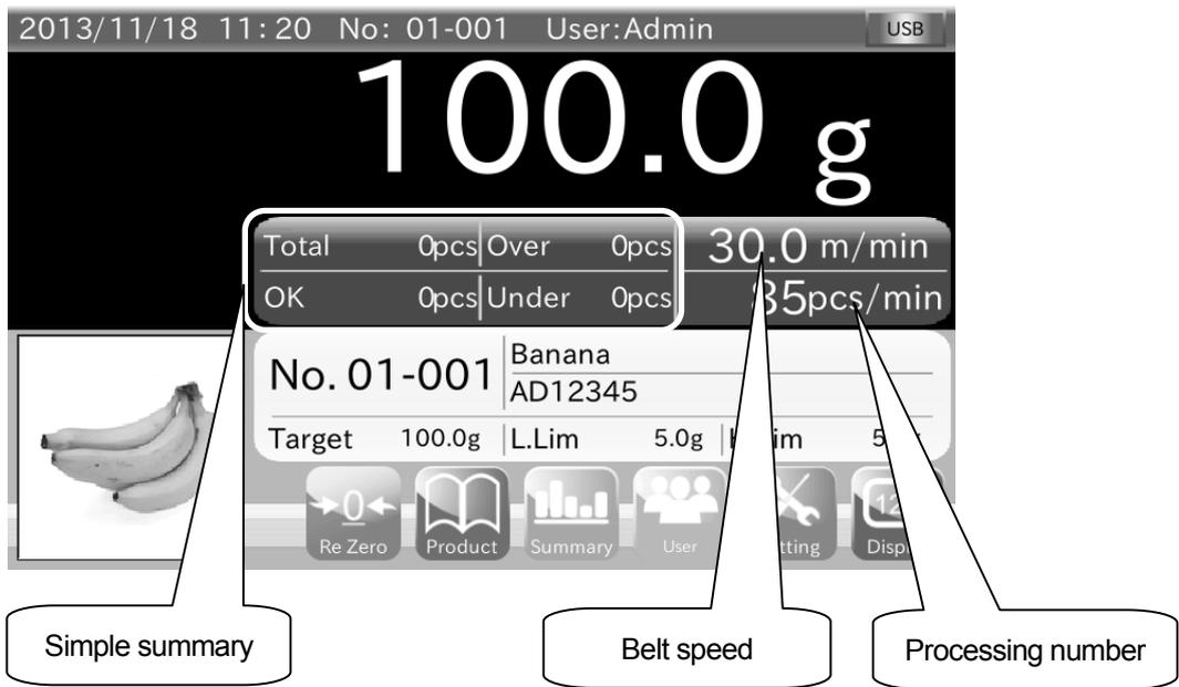
**Fig.14 Display example (Reduced regular display)**
