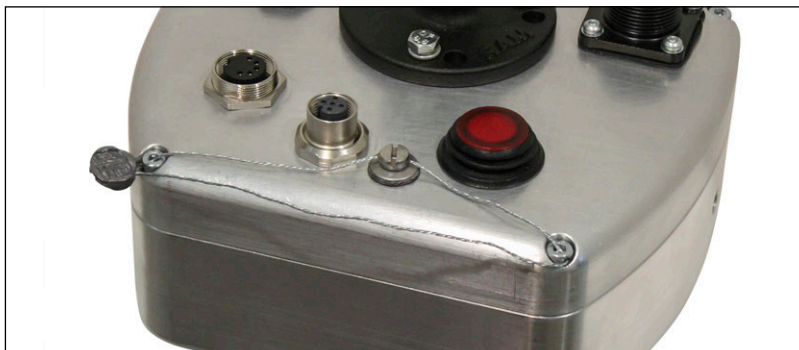
Figure 2-12. Sealing the Enclosure – No Access
