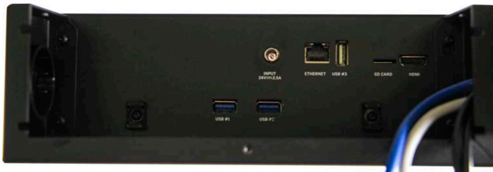
Figure 3-3. Feed Cables Through Head
