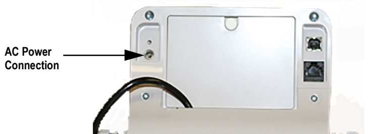
Figure 2-5. Power Connection Site
